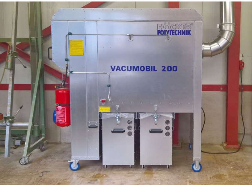
Illustration below: Vacumobil VT 200 with fire suppression system (optional)
